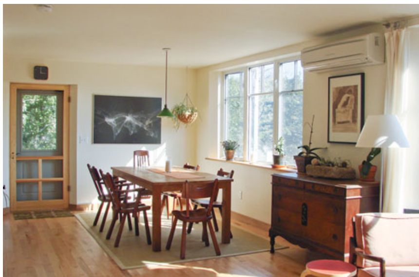
Figure 11. The insulation and air-barrier systems are so effective that a single mini-split heat pump should be able to provide heating and cooling for the entire home. Electric radiant ceiling panels will provide backup heat if needed.
